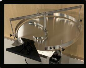
Surge Tables are engineered to accumulate round bottles or containers along a production line in case of line backup or stoppage. Containers are guided from a conveyor onto the table and flow back onto the conveyor line.
