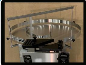
Accumulation Tables are engineered to collect round bottles or containers at the end of a production line. Containers are guided from a conveyor onto the stainless steel table top.
